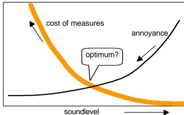
**Figure 3** The reduction of annoyance asks for additional reduction of vibrations with measures. This will add costs to the project. The question is to find an acceptable annoyance level for reasonable costs.
