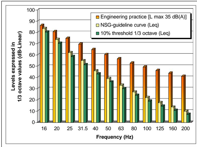
**Figure 4** Soundlevels for threshold of hearing (10% group) and NSG-guideline expressed in 1/3 octave band levels. The Lmax 35 dB(A) value (engineering practice see section 3.3) is added as reference and expressed in 1/3 octave bands assuming that the level is determined by the level in one octaveband (correction of -5 dB re 35 dB(A)).
